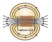
The pattern of the magnetic field lines around a current-carrying solenoid
