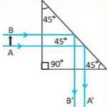
Statement 3: Optical fingerprinting devices use frustrated total internal reflection in order to record an image of a person's fingerprint without the use of ink.
