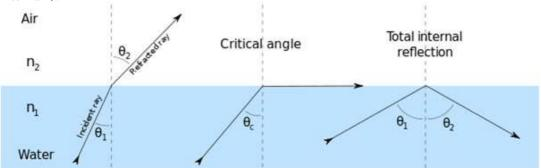
**Justification:** Statement 1: Optical fibres, which are widely used in telecommunications, keep the signal reflected within the fibre using total internal reflection.
